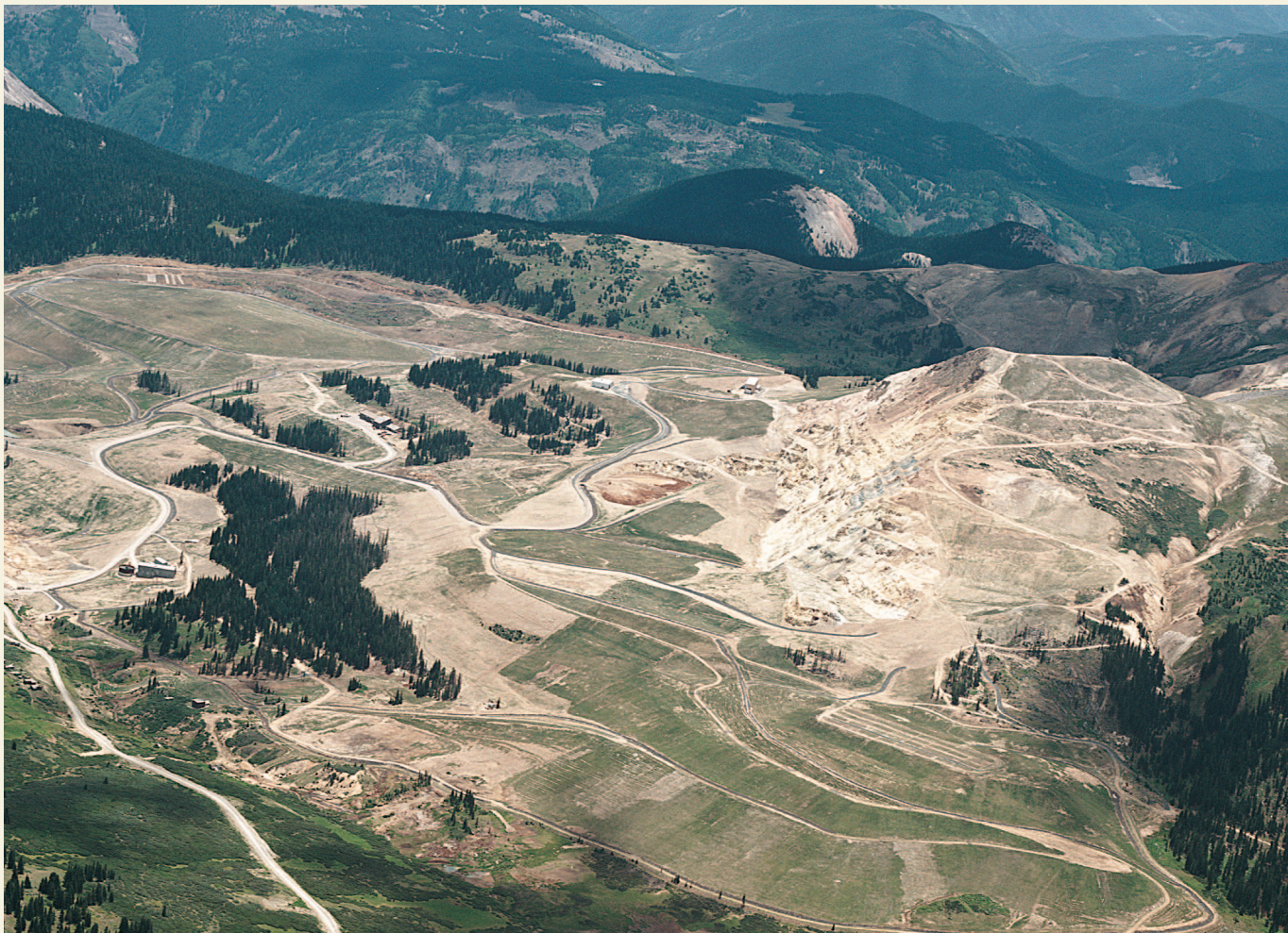
Scar tissue. A crisscross of roads and pits scars the surface of a former gold mine in Summitville, Colorado, while underground workings and tunnels allow acidic waste to drain into nearby watersheds. The Superfund site has cost more than $150 million in remediation efforts and remains incomplete.
