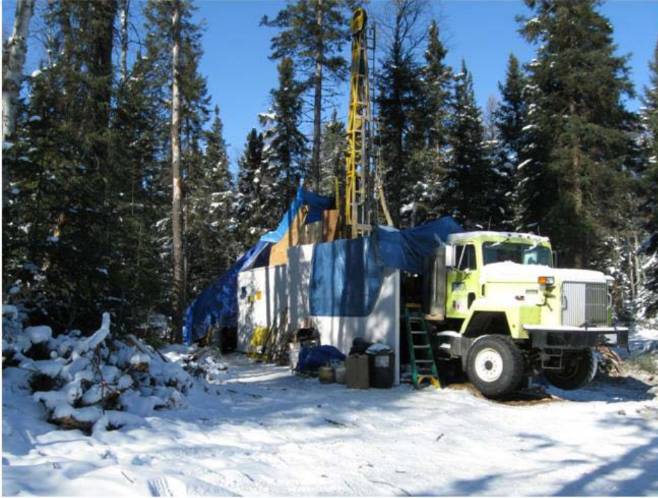
Figure 4. Truck mounted drill rig
